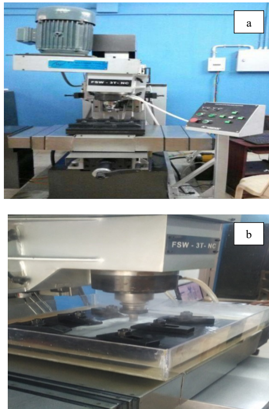
Figure 1. a) Normal FSW experimental setup. b) Submerged FSW experimental setup.
