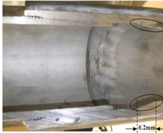
Figure 10 Axial erosion length test (erosion time is 55 h)
