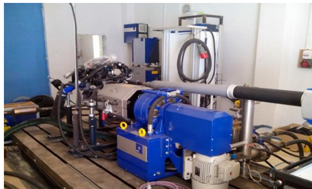
Figure 1. View of the engine test bench (Seddak et al., 2018).
