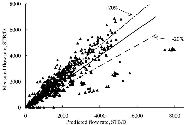
**Fig. 2.** Measured and predicted values with  $\pm 20\%$  scatter lines (dashed) for the choke correlations without considering API gravity as influencing parameter.
