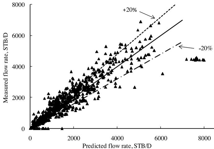
**Fig. 3.** Measured and predicted values with  $\pm 20\%$  scatter lines (dashed) for the choke correlations with employment of API gravity.
