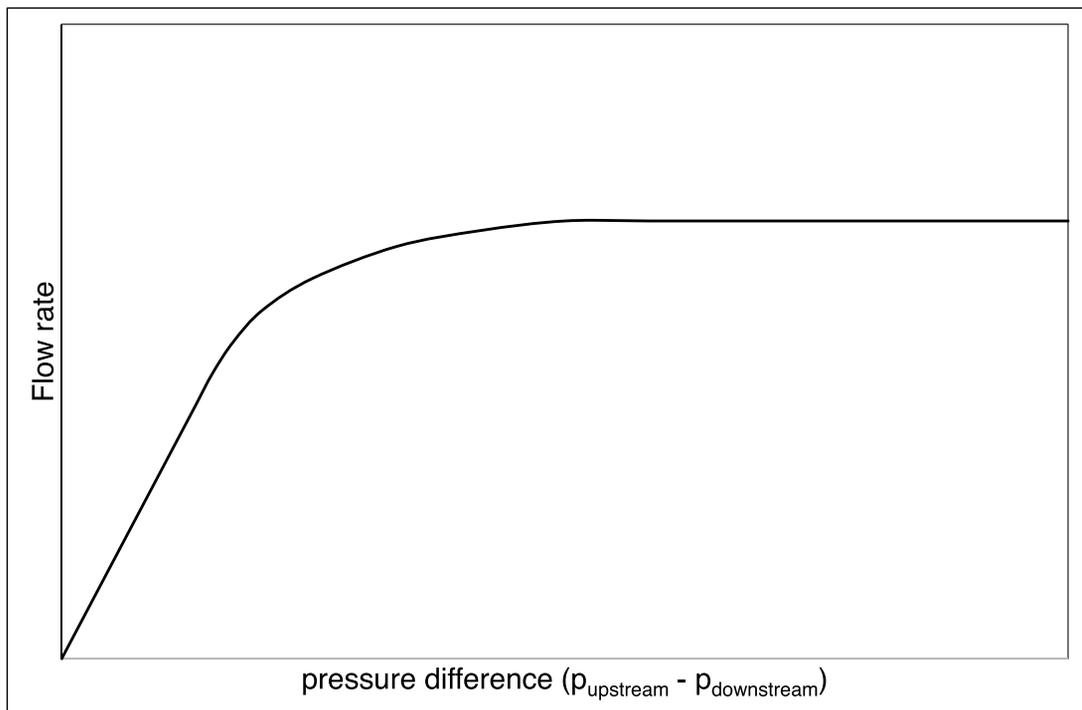
**Fig. 1.** The flow rate behaviour vs. pressure difference.
