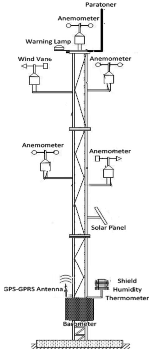
**Figure 2.** Wind speed/solar radiation measuring station.
