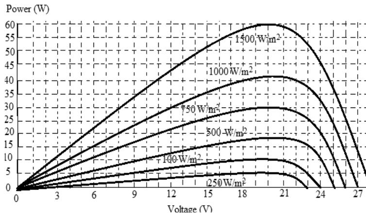
**Figure 9.** Voltage-power curve of 2 kW solar panels.
