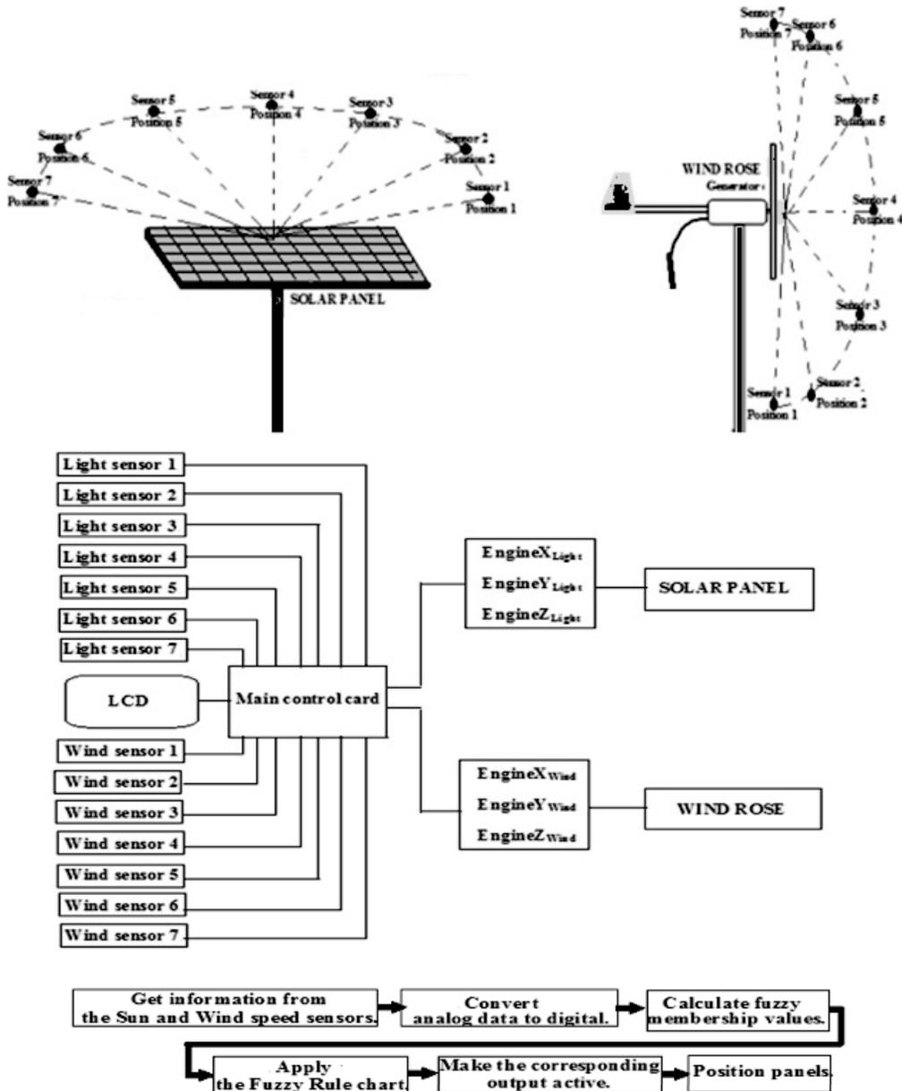
Figure 6. System diagrams of tracing the direction of the sun and the wind.
