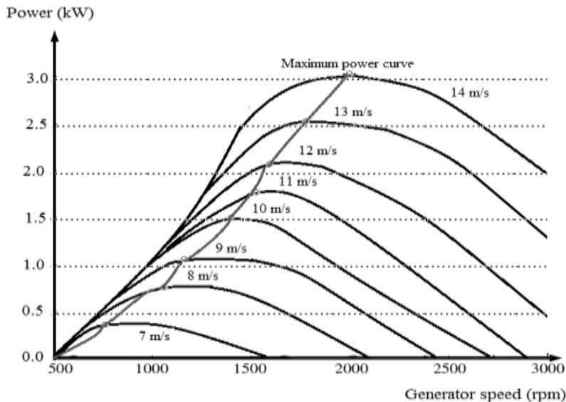
**Figure 10.** Speed-power curve of a 5 kW wind turbine.
