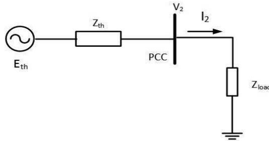
**Figure 7.** Equivalent Thevenin circuit for an integrated AC/DC grid.
