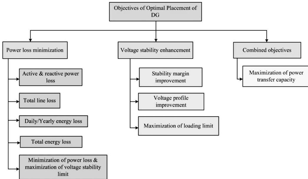
**Figure 3.** Classification of optimal DG placement objectives.
