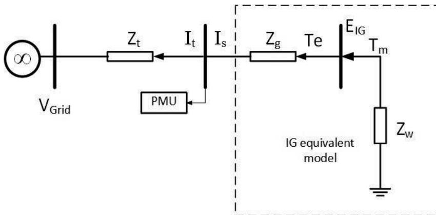
Figure 4. The equivalent model of FSIG connected to the grid.
