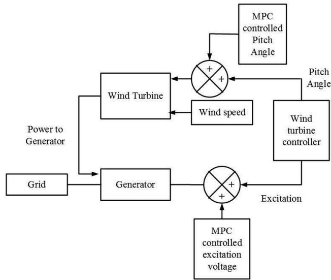
**Figure 9.** Model predictive control used in a wind turbine system.
