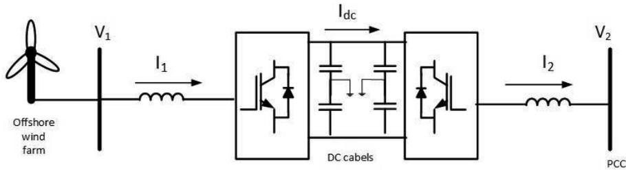
Figure 5. VSC-HVDC connected wind farm.
