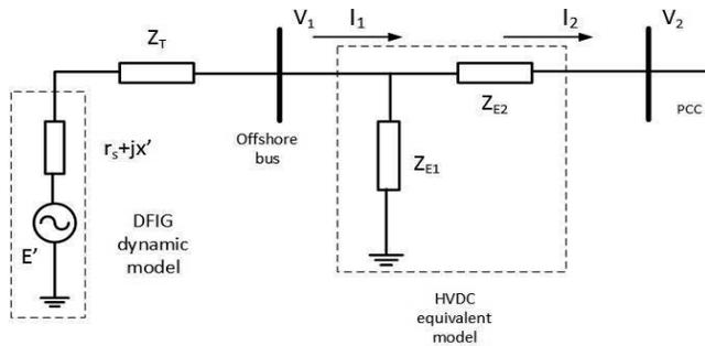
Figure 6. Equivalent model of HVDC connected offshore wind farm.
