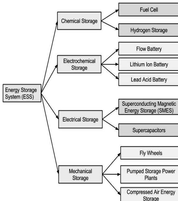
**Figure 10.** Energy storage systems used in renewable energy systems.
