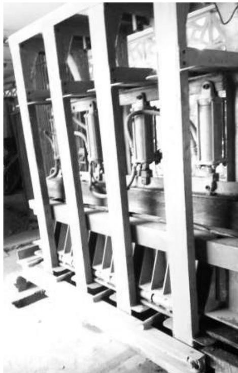
**Fig. 6.** Mechanized System for compression and consolidation of earth blocks.
