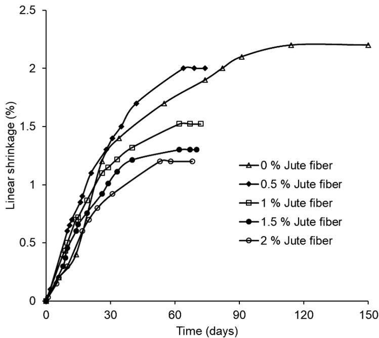
**Fig. 16.** Effect of jute fiber on linear shrinkage of compressed earth blocks.
