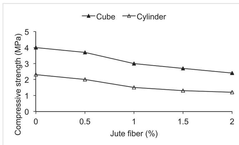
**Fig. 13.** Effect of dosage of jute fiber on compressive strength of cubes and cylinders.
