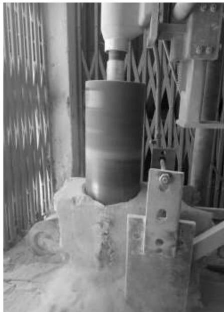
**Fig. 9.** A cylinder is being cut from a portion of Compressed Earth Block.
