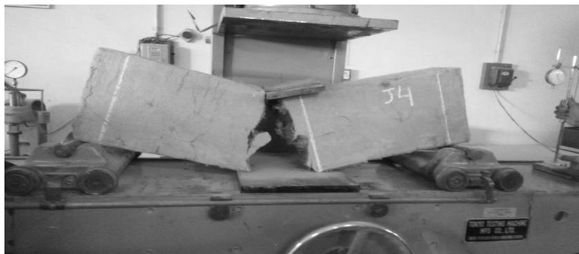
Fig. 15. Flexural mode of failure of a Compressed Earth Block reinforced with 2% jute fiber.
