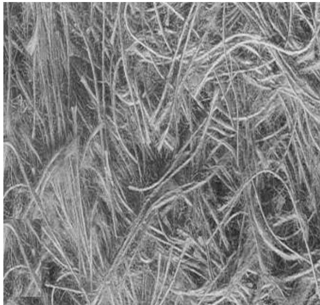
**Fig. 4.** Jute Fiber chopped from old gunnysacks.
