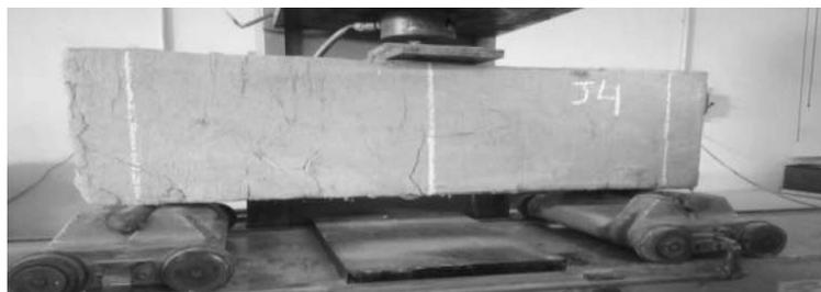
**Fig. 12.** A Compressed earth block is being tested for modulus of rupture in Universal Beam Testing Machine.
