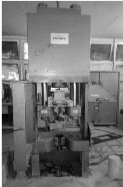
**Fig. 10.** Cube crushing strength is being performed in Universal Testing Machine.
