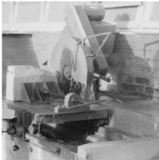
**Fig. 8.** Cutter machine utilized for sawing cubes from Compressed Earth Blocks.
