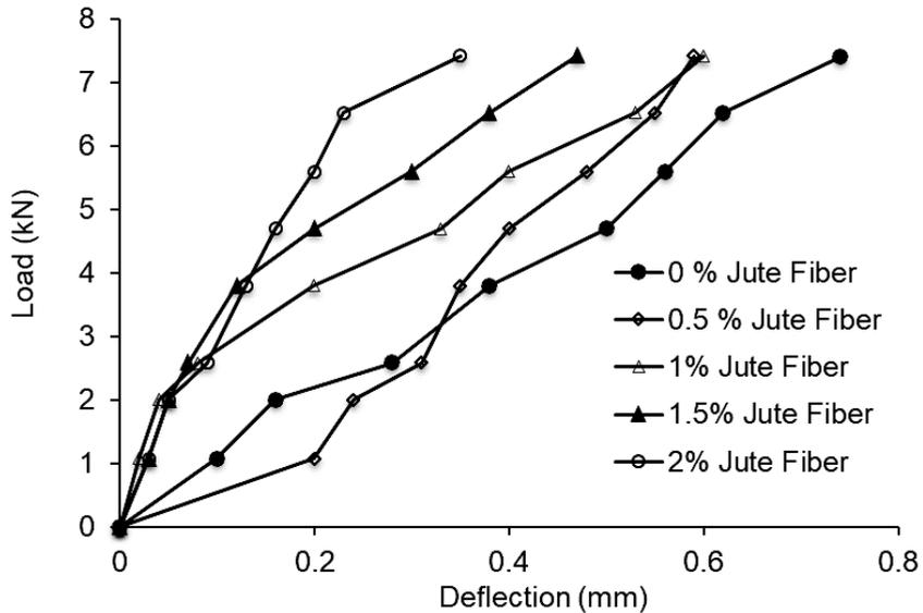
Fig. 14. Effect of jute fiber content on load deflection behaviour of compressed earth blocks.
