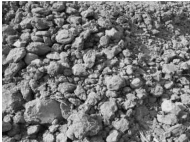
**Fig. 1.** Excavated clay in form of lumps.
