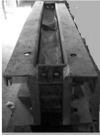
**Fig. 5.** Mould for casting earth blocks.
