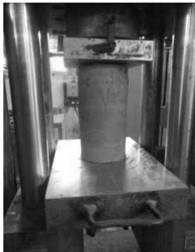
**Fig. 11.** A cylinder cut from a compressed earth block is being tested for compressive strength in Universal Testing Machine.
