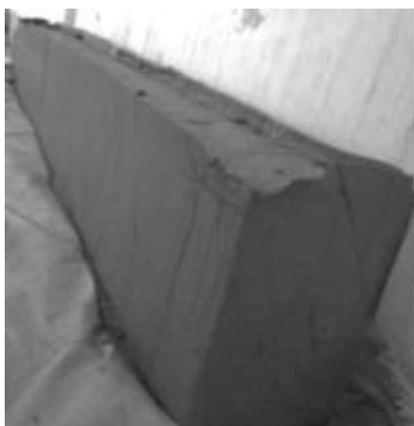
**Fig. 7.** A Compressed Earth Block is being dried in shade.
