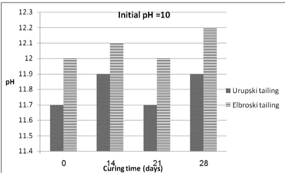
Fig. 8. Change of leachate pH value with curing time for samples with initial pH of 10.
