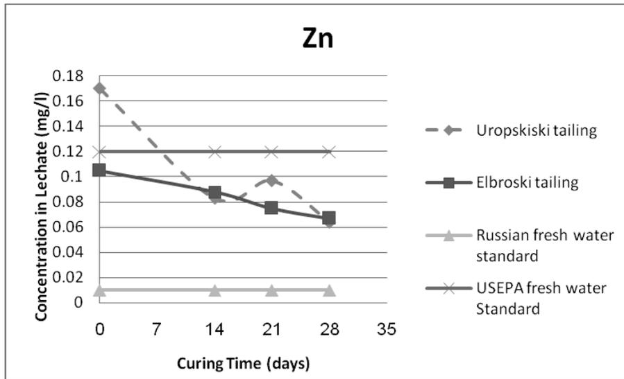
**Fig. 4.** Zinc concentration in leachate from solidified Urupsky and Elbrosky tailings as compared to Russian and USEPA standards.
