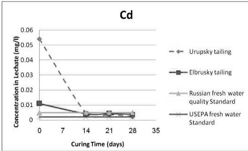
Fig. 2. Cadmium concentration in leachate from Urupsky and Elbrusky tailings as compared to Russian and USEPA standards.
