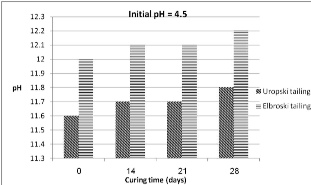
Fig. 6. Change of leachate pH value with curing time for samples with initial pH of 4.5.
