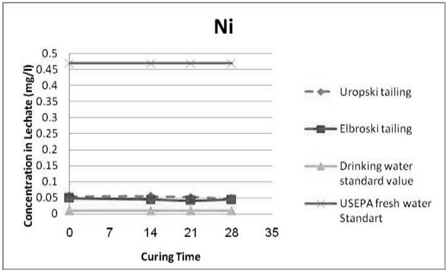
Fig. 5. Nickel concentration in leachate from solidified Uropiski and Elbroski tailings as compared to Russian and USEPA Standards.
