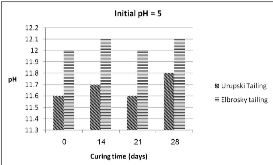
Fig. 7. Change of leachate pH value with curing time for samples with initial pH of 5.
