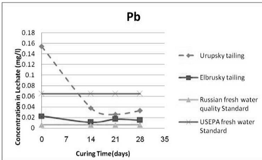
Fig. 3. Lead concentration in leachate from solidified Urupsky and Elbrusky tailings as compared to Russian and USEPA standards.
