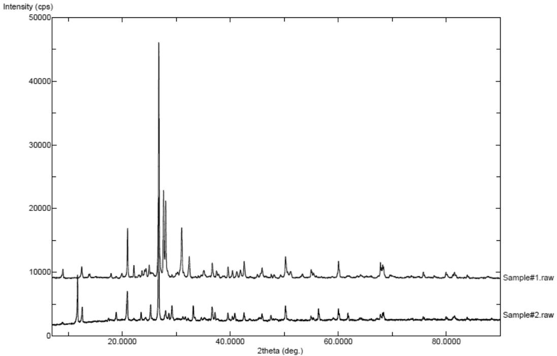
**Fig. 1.** XRD patterns of both Urupsky (sample 1) and Elbrosky (sample 2) tailings.
