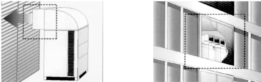
**Fig. 2.** Outdoor units of VRF air conditioner with arced exhaust hood.
