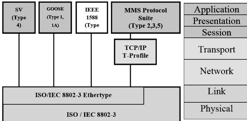
Fig. 1. Mapping of messages as per IEC 61850 standard.
