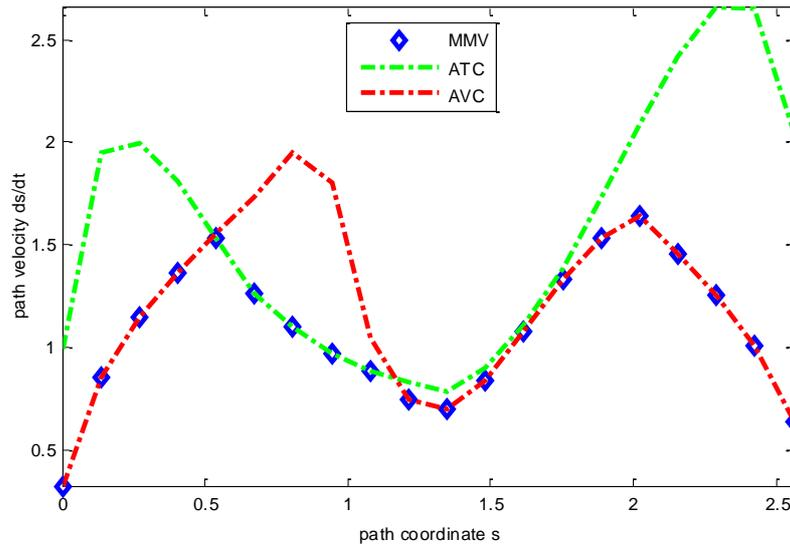
**Figure 3.** The schematic of three kinds of constraints speed curve.
