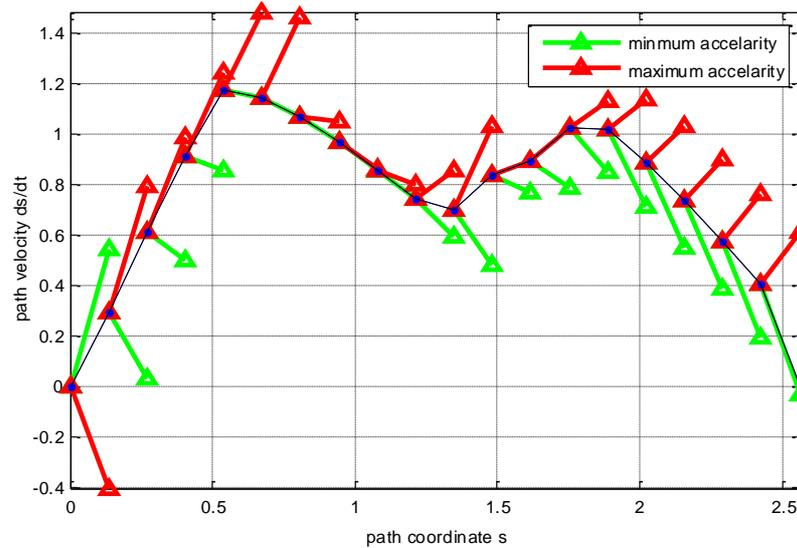
**Figure 7.** The velocity distribution diagram after velocity sinking approach.
