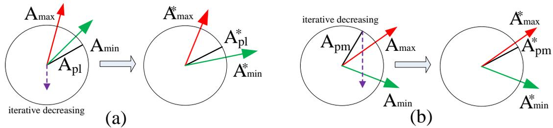
**Figure 6.** The velocity distribution diagram after velocity sinking approach The velocity profile in the Velocity Sinking approach ((a) represents the actual acceleration is less than the minimum constraint acceleration, (b) represents the actual acceleration is greater than the maximum constraint acceleration).
