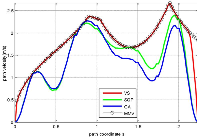
**Figure 9.** The path velocity of different planning method.
