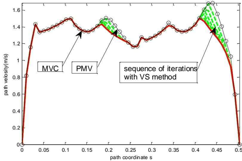
**Figure 13.** The schematic of VS method.
