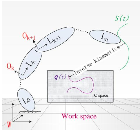
**Figure 1.** A schematic of time-optimal trajectory planning with path constraint.
