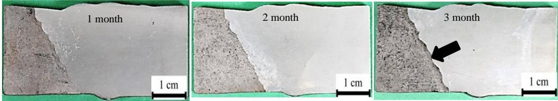
Figure 4. Observe the macroscopic surface of the A508/IN-182/316L specimen after immersion
