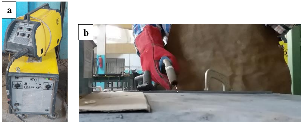
Figure 2. (a) Welding machine CEA MAXI 321, (b) Welding process.
