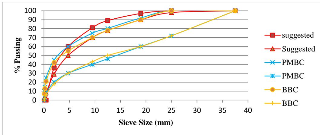
**Figure 3.** Comparison of gradation recommended for FBSM with PMBC and BBC gradations
