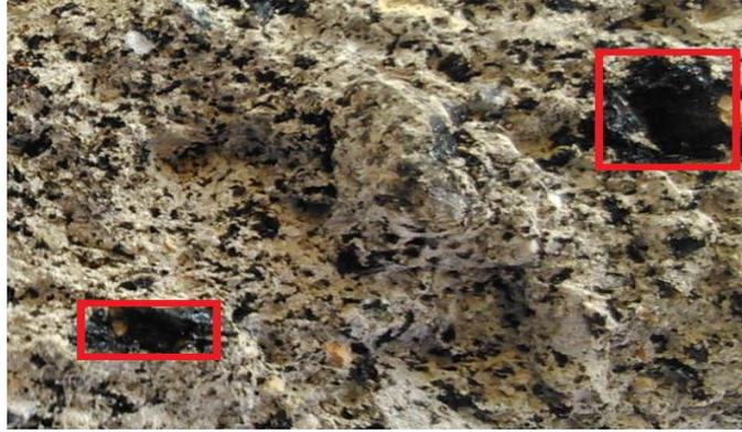
**Figure 1.** Different distribution regions of bitumen in the briquette internal structure
