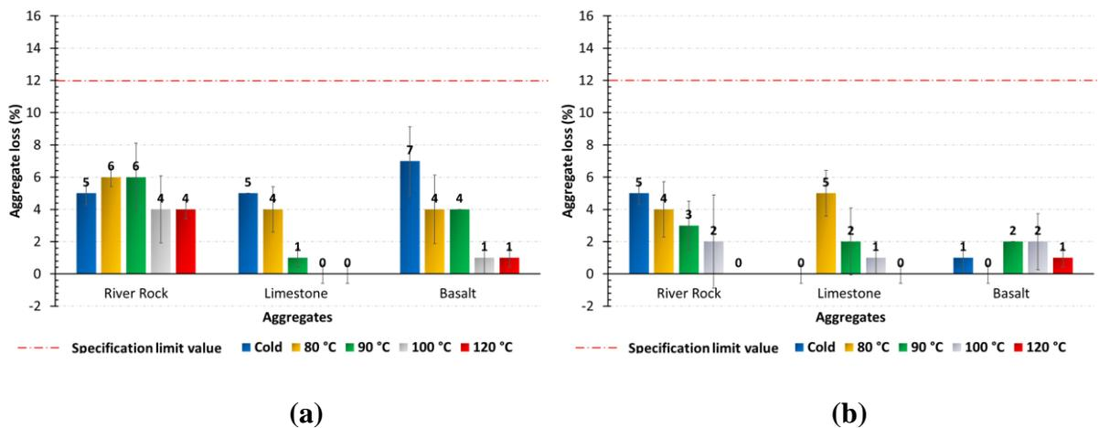
**Figure 1.** Vialit adhesion test results (a) unmodified B50/70, (b) unmodified B160/220 binders.
