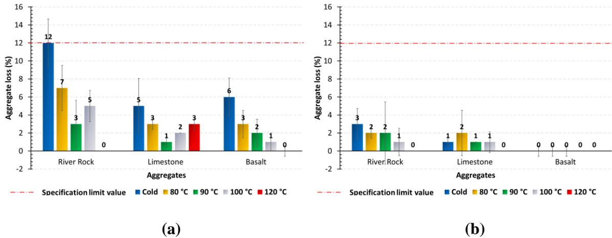
**Figure 2.** Vialit adhesion test results; (a) B50/70 binder with 1% PPA, (b) B160/220 binder with 1.1% PPA.
