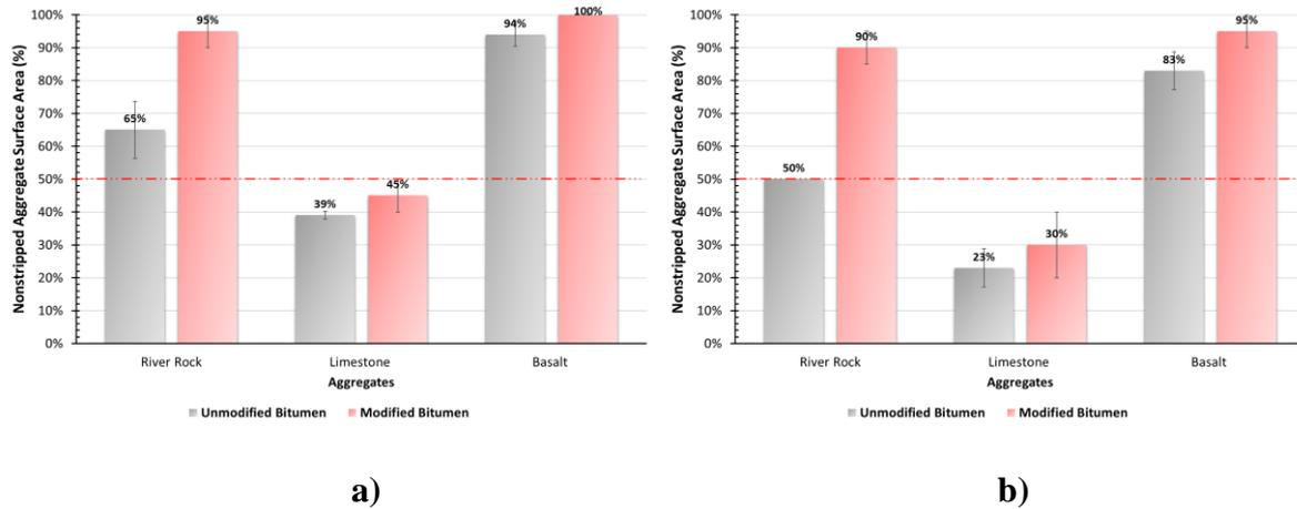
**Figure 3.** Nicholson stripping test results; a) B50/70 binder, b) B160/220 binder.
