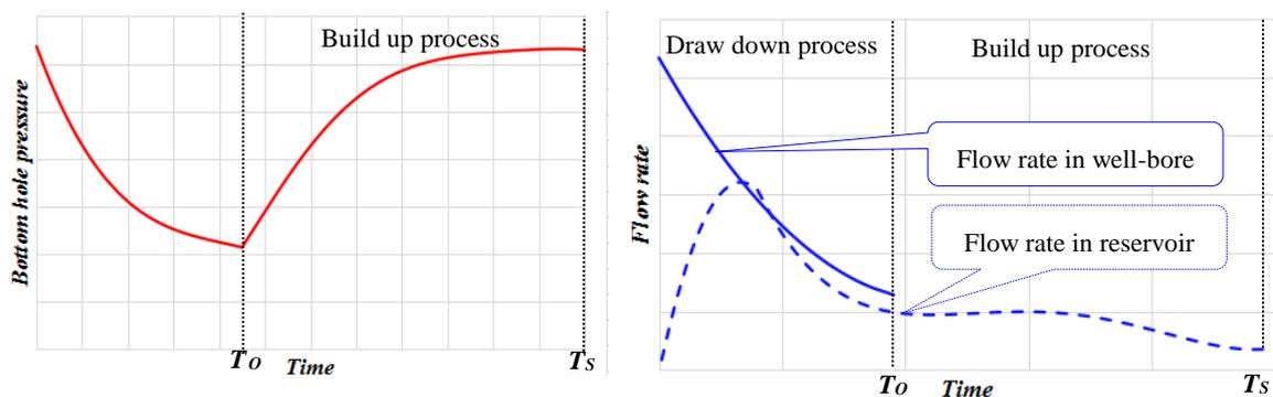
Figure 1 Variation of bottom-hole pressure and flow rate in low pressure gas wells
