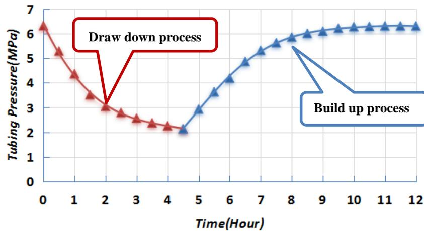
Figure 5 Variation of the tubing pressure in one period of production
