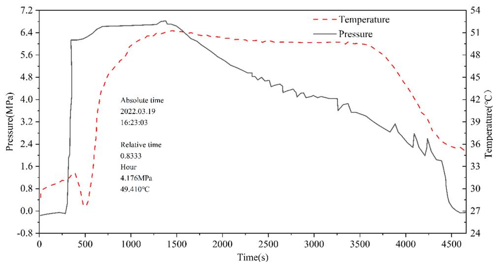
Figure 3 Pressure variation of the gas well when it starts to produce gas
