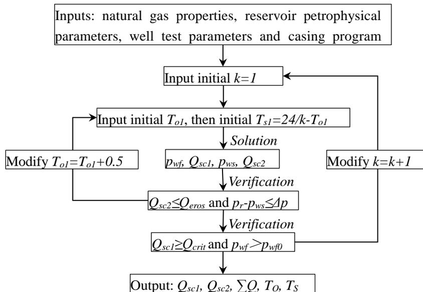
Figure 2 Flow scheme for producing period calculation
