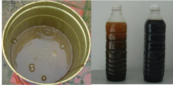
Figure 4 Liquid samples lifted out from the gas well
