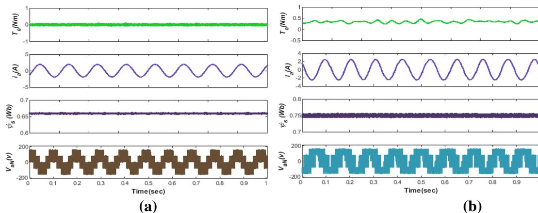
**Figure 9.**  $L_m$  mismatch analysis at no-load rated speed a) FCS-MPFOC b) MPTC
