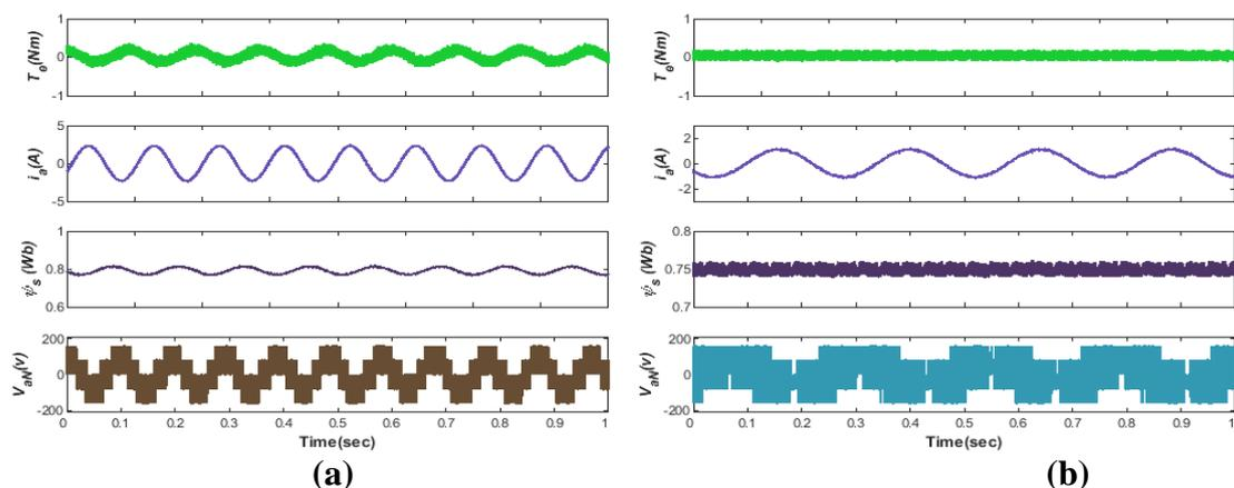
**Figure 7.**  $R_s$  sensitivity analysis at zero-load under rated speed **a)** FCS-MPFOC **b)** MPTC
