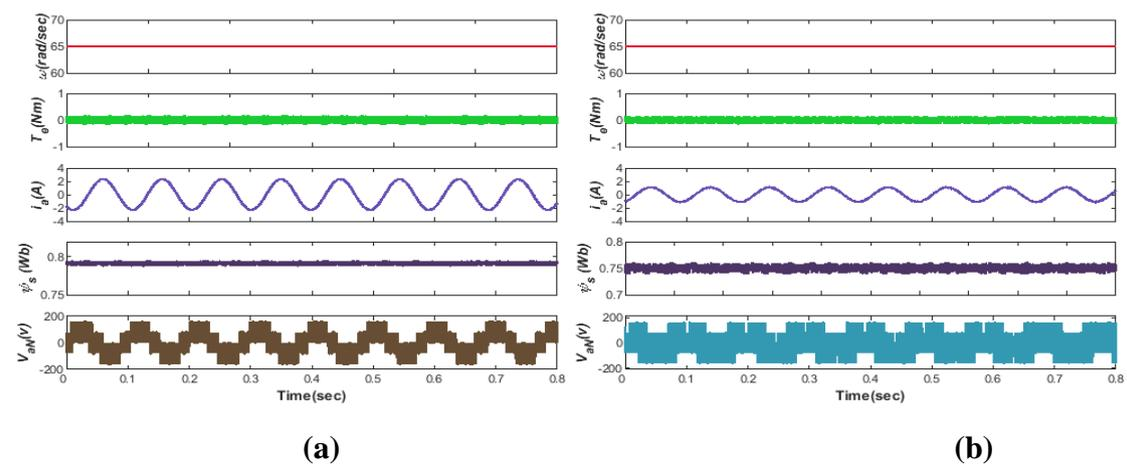
**Figure 5.** Steady-state analysis at rated speed **a)** FCS-MPFOC **b)** MPTC
