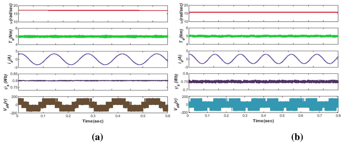
**Figure 6.** Performance validation at low speed a) FCS-MPFOC b) MPTC
