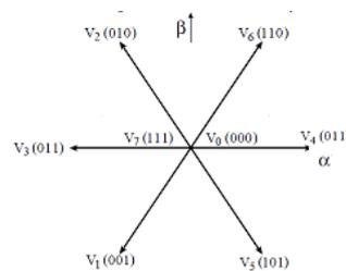
FIGURE 1b- 2L-VSI output voltage vector's
