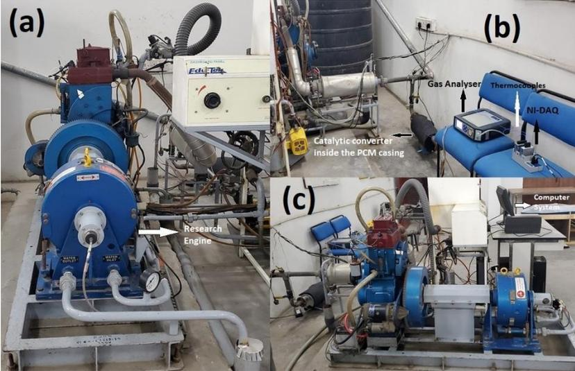
Figure 2: (a) Research Engine side view, (b) Experimental Setup, and (c) Front view of the Research Engine.
