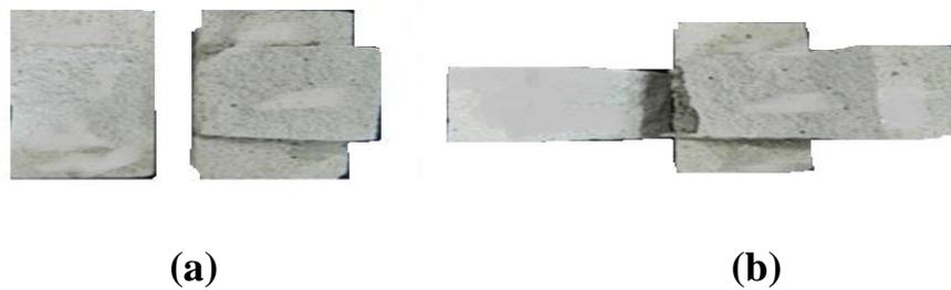
**Figure8:** (a) Incomplete block-mortar block (Type-II) interface failure, (b) tensile failure of the whole block (Type IV)
