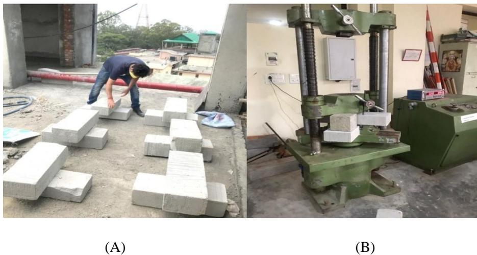
**Figure7:** (A) cross-couplet samples, (B) tensile bond strength
