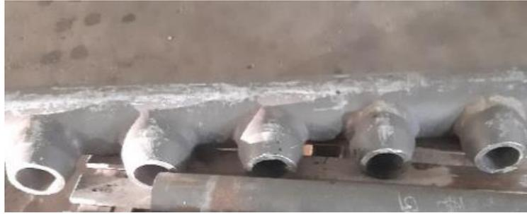
**Figure 1.** Outlet Manifold Bottom Header
