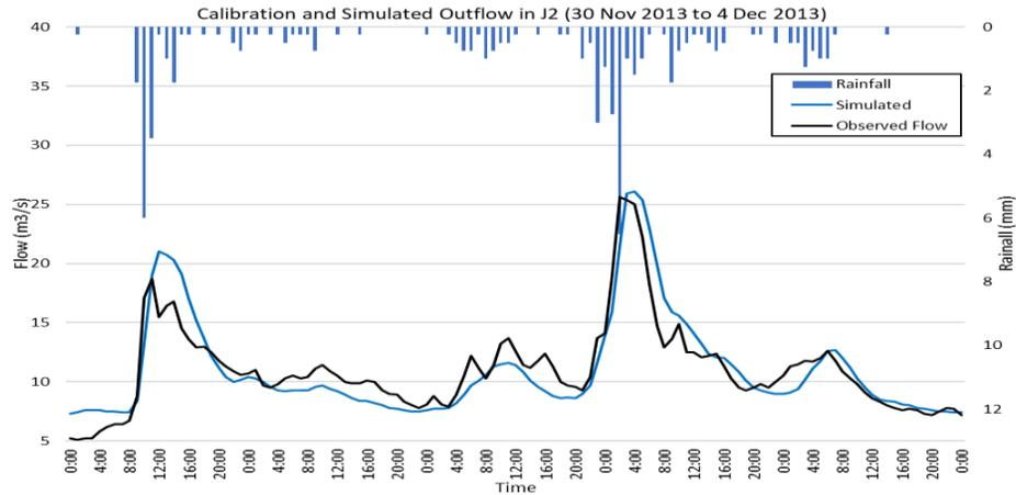
**Figure 5.** The Calibration Hydrograph
