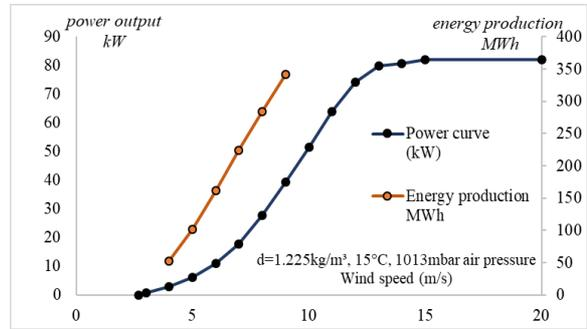
**Figure 6.** The energy production curve and the power-speed curve of the wind turbine
