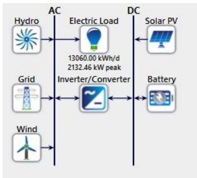
**Figure 8.** Schematic diagram of the on-grid hybrid system
