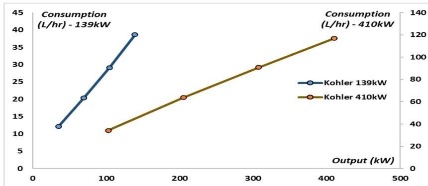
**Figure 7.** The fuel consumption curve of diesel generators
