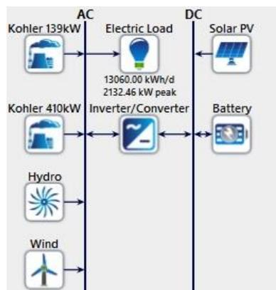
**Figure 10.** Schematic diagram of the off-grid hybrid system
