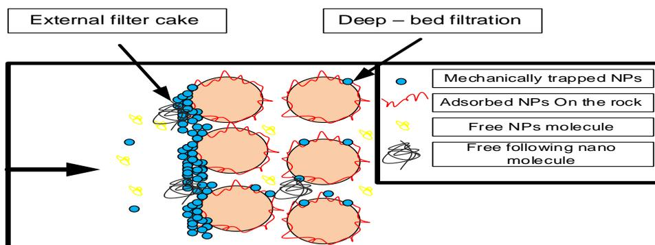
**Figure 3** Deep bed formation and external cake formation for NPs around the wellbore.
