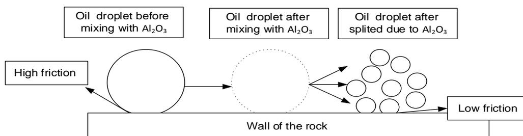
**Figure 1**  $\text{Al}_2\text{O}_3$  mechanism to reduce oil viscosity.
