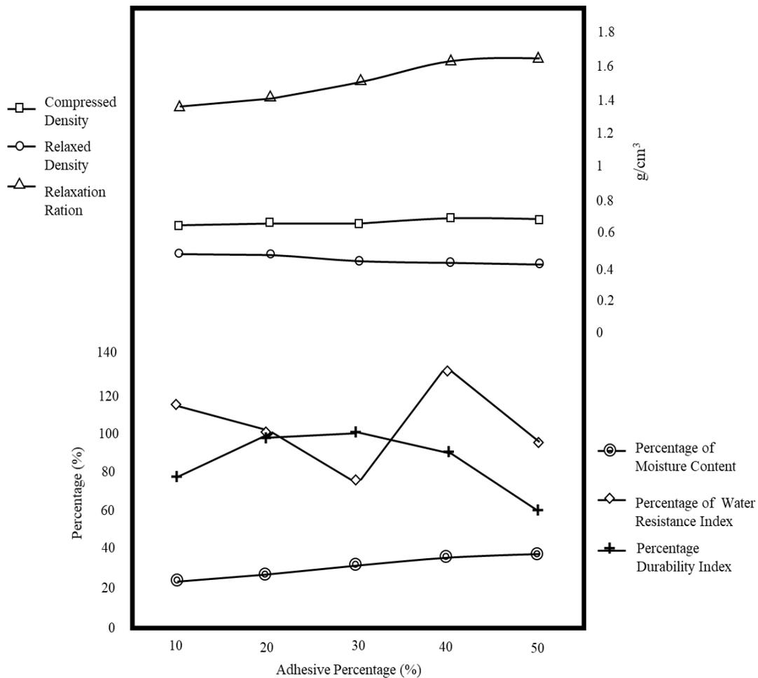
**Figure 2** Graph of CD, RD, RR, PMC, PWRI, and PDI test results with variations in the composition of rice adhesives 10, 20, 30, 40, and 50%. Example of figure
