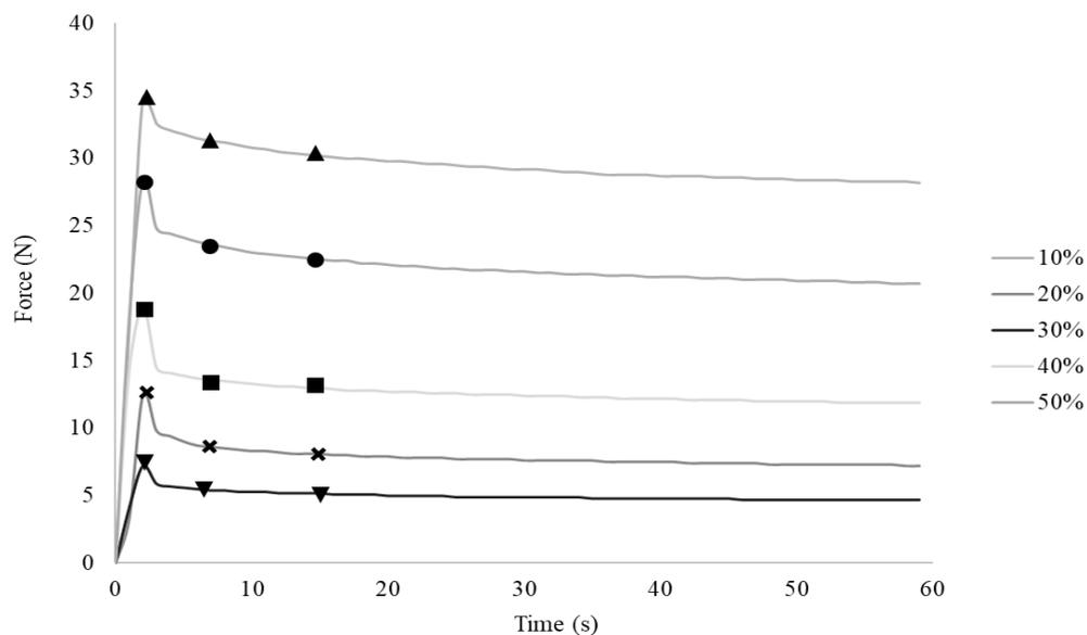
**Figure 4** The hardness test results with variations in the composition of rice adhesives.
