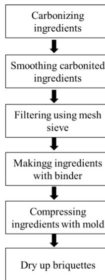
**Figure 1** Briquettes making mechanism
