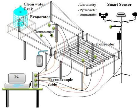
**Figure 1** Schematic of single slope desalination
