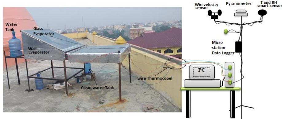
**Figure 3** Experimental equipment and data acquisition systems
