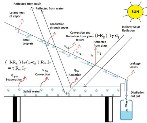
**Figure 2** Heat transfer scheme of single slope desalination
