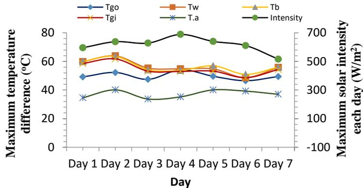
**Figure 4** Day variation of maximum temperature difference, among the solar intensity and overall temperature
