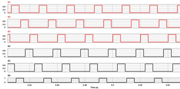
**Figure 4.** TCR gate signals waveform ( $146.65^\circ$  triggering angle)
