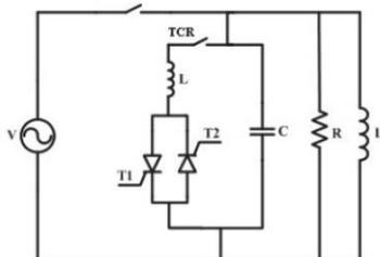
**Figure 1.** A simplified model of single FC-TCR compensator
