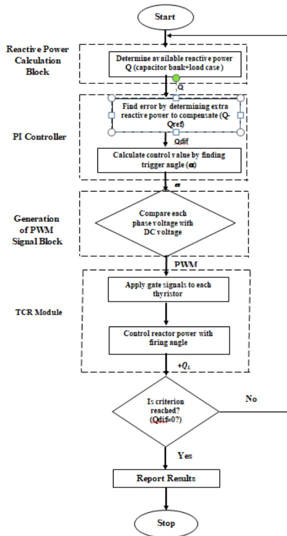
**Figure 2.** Flowchart of FC-TCR based compensation system
