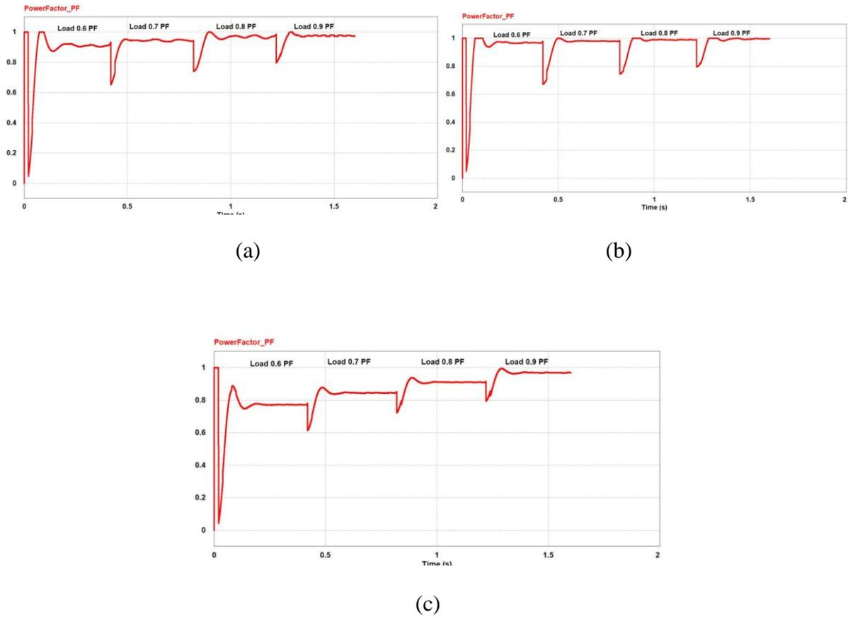
**Figure 12.** Power factor under variable load with P controller ( $K_p=0.04$ ) (a), PI controller ( $K_p=0.04$ ,  $K_i=100$ ) (b) and PID controller ( $K_p=0.04$ ,  $K_i=100$ ,  $K_d=0.01$ ) (c)
