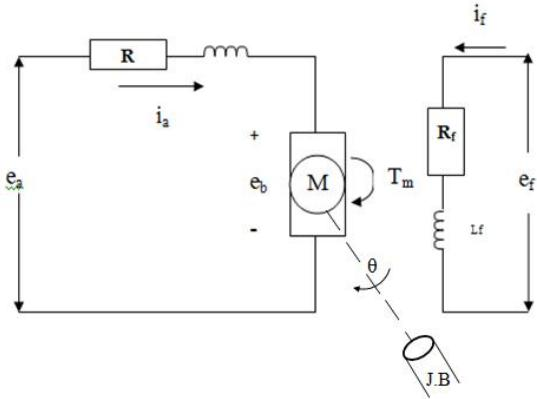
**Figure 1** Separately excited constant field current DC Motor
