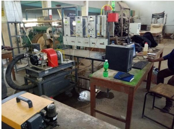
**Figure 1. Experimental setup for the performance and emission test analyzer setup**
