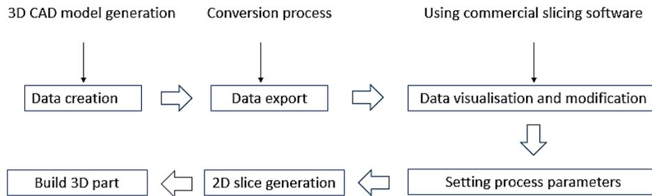
**Figure 1** General steps in Additive Manufacturing process
