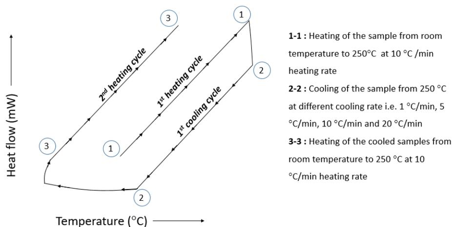
**Figure 2** DSC procedure for 250° C specimen
