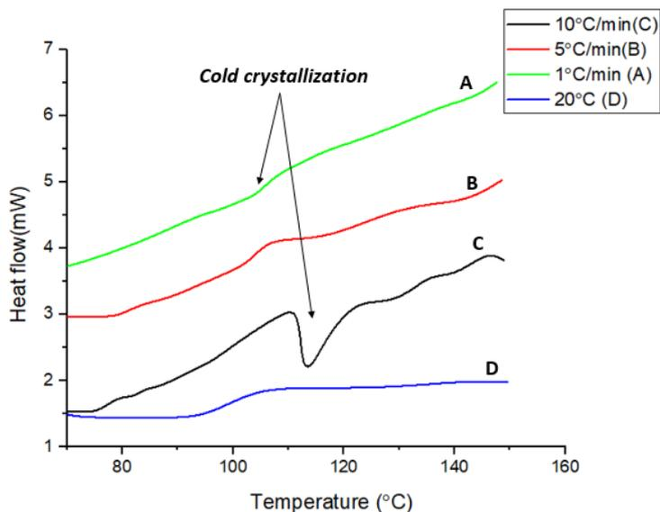
**Figure 3** DSC testing curve 2<sup>nd</sup> heating cycle (for the part manufactured at 250° C extruder temperature)
