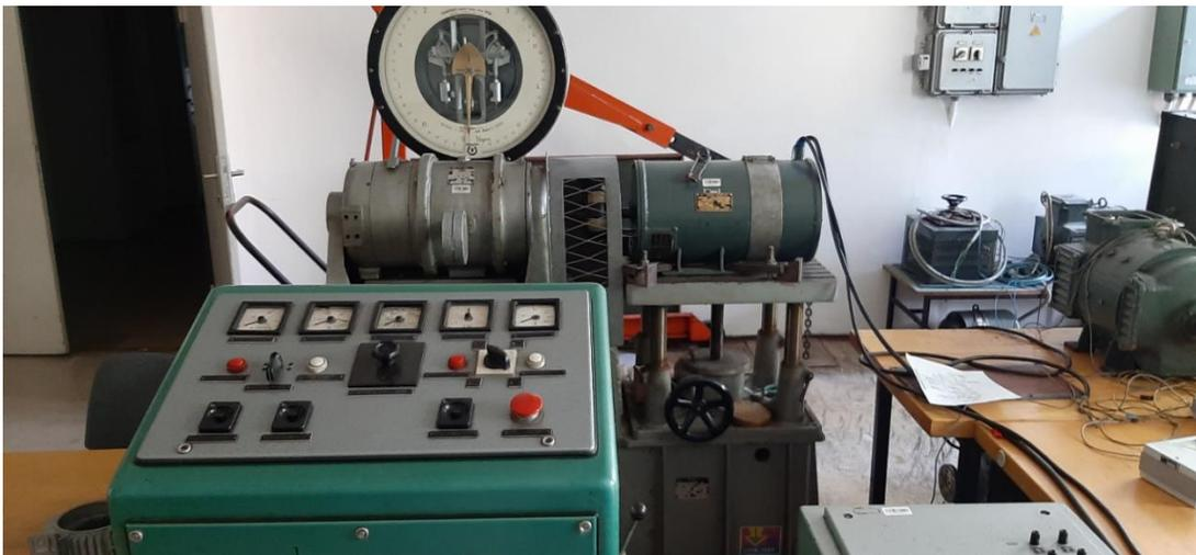
**Figure 7** Hardware structure used to accurately measure load angle
