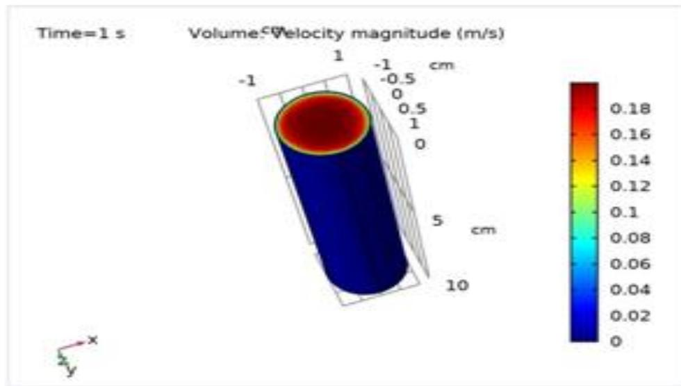
**Figure 5.** Laminar flow of Working fluid showing flow rate is maximum in the middle of any cross-section
