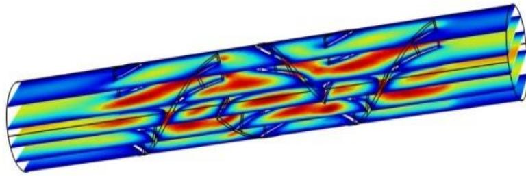
**Figure 8.** Particle tracing inside a pipe: Velocity of particles at different layers
