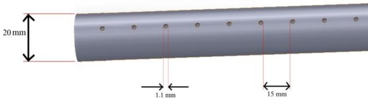
**Figure 4** Series of 1.1mm holes (nozzle) in a pipe with a gapping of 15mm.
