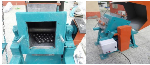
Figure 3. Impact Resistance Test Device
