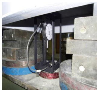
Figure 4 Measurement of deformation in slab samples
