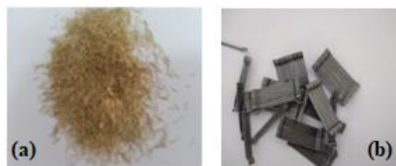
Figure 1 (a) Brass coated micro steel fiber and (b) macro steel fiber
