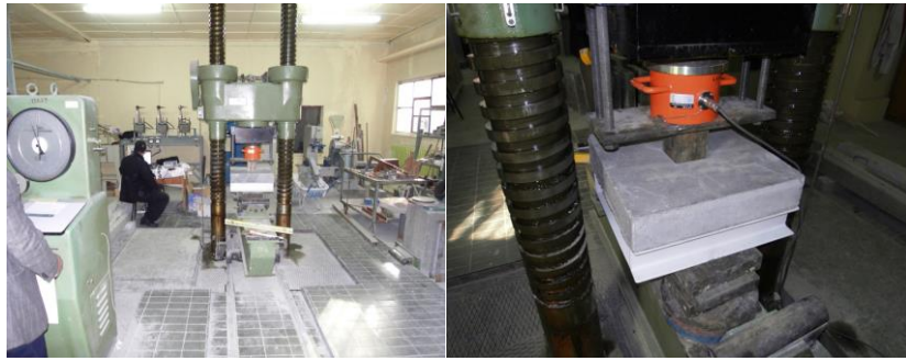
Figure 2 The testing of slab samples
