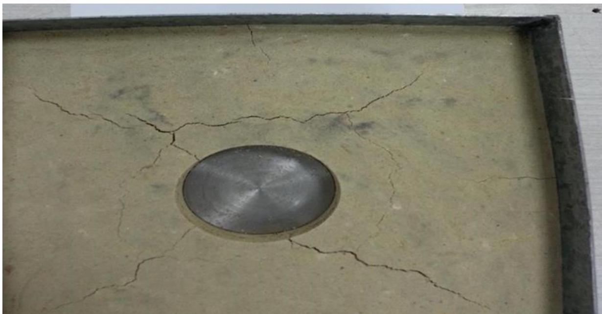
Figure 6b After failure view showing punching failure and radial cracks
