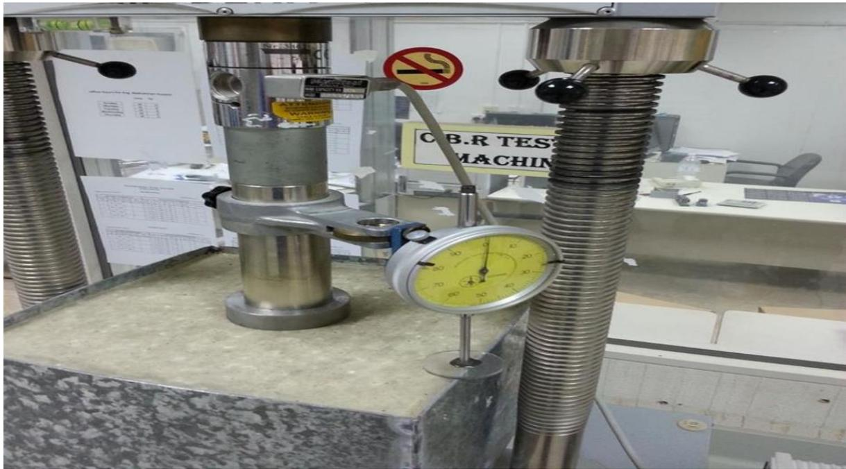
Figure 6a Load test set up on clayey sand (gatch) soil
