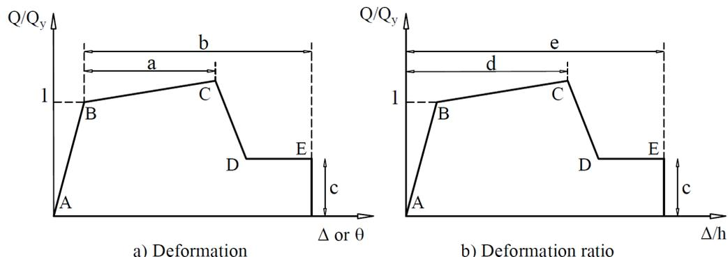
**Figure 2.** Generalized force-deformation relationships for concrete elements or components
