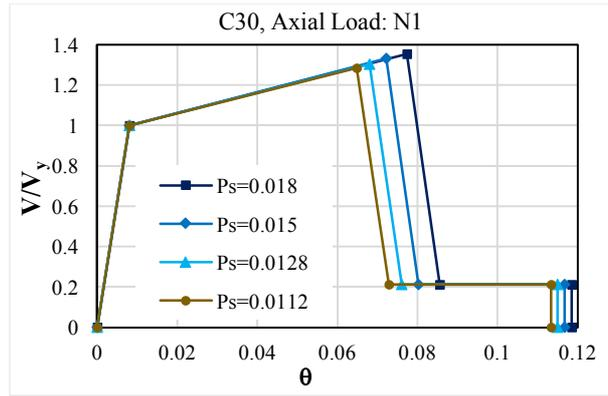
**Figure 3.** Generalized force-deformation relationship according to ASCE/SEI-41 (2017)
