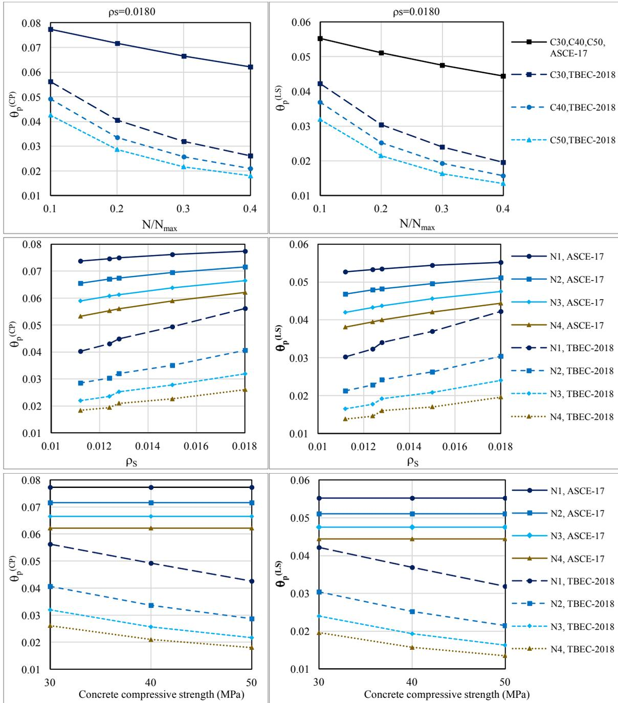
**Figure 4.** Comparison of deformation limits for different performance levels
