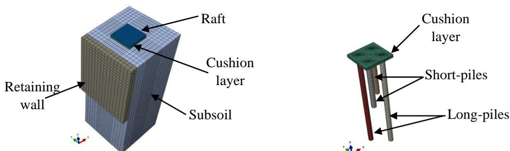
**Fig. 6.** The 3D and internal view of FE mesh of the composite foundation and retaining wall
