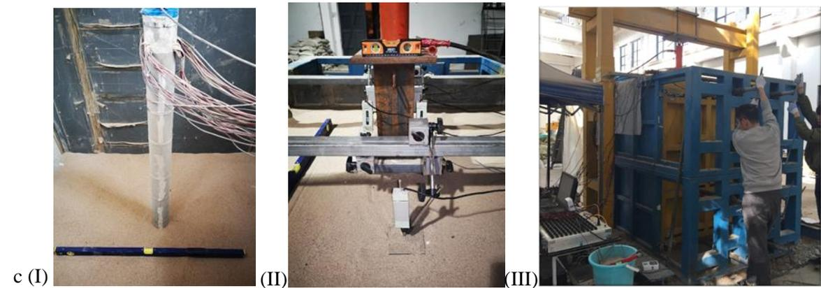
**Fig. 1.** Schematic view of the test model set-up: a) sectional view (section A-A), b) plan view, c) photographs taken during (I) instrumented pile embedment, (II) raft & hydraulic jack placement on top of the cushion, and (III) wall rotation
