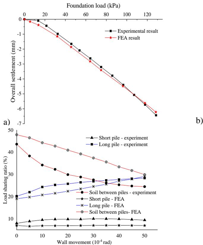
**Fig. 7.** Comparison of experimental (a) load settlement curve and (b) load sharing ratio during wall rotation with finite element analysis result
