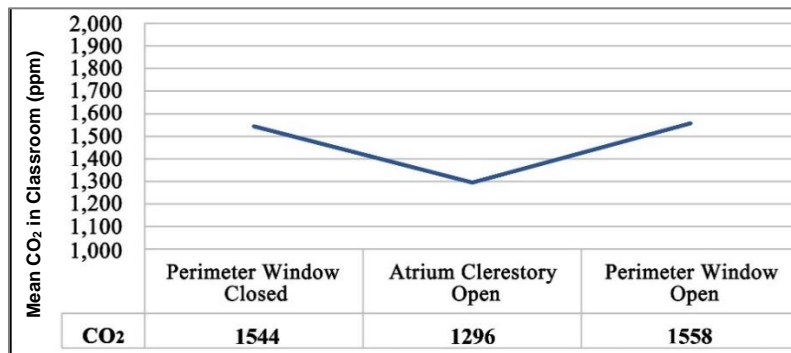
Figure 9. Classroom CO 2 concentration levels according to window positions in pilot central AC classrooms.
