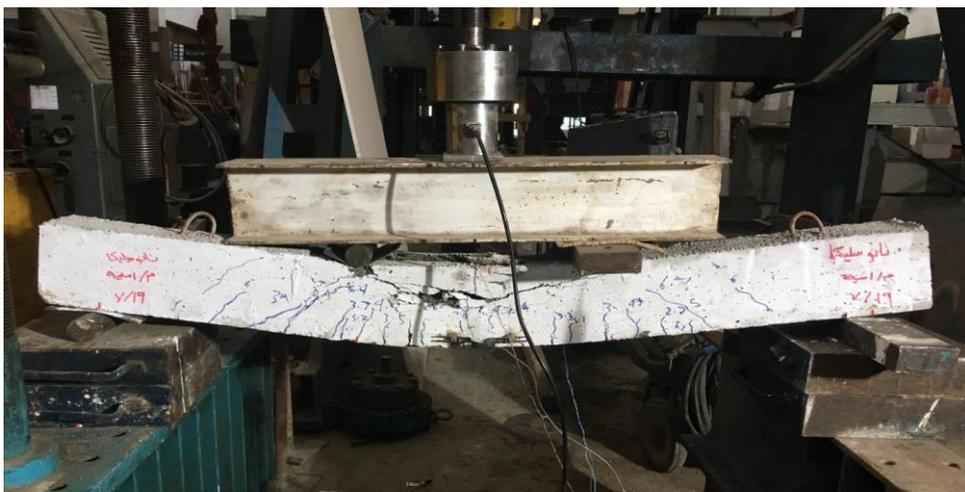
Figure 8 Failure of 0.75% NS concrete beam
