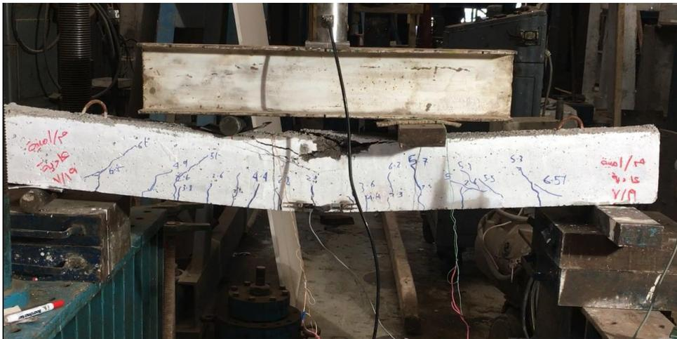
Figure 7 Failure of normal concrete beam under flexure
