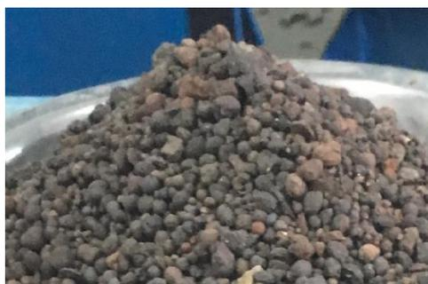
Figure 3 Locally produced LECA used in this study
