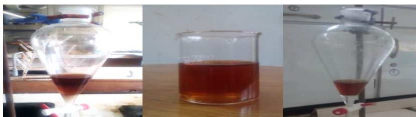
Figure 1. Phase separation and purification of biodiesel.
