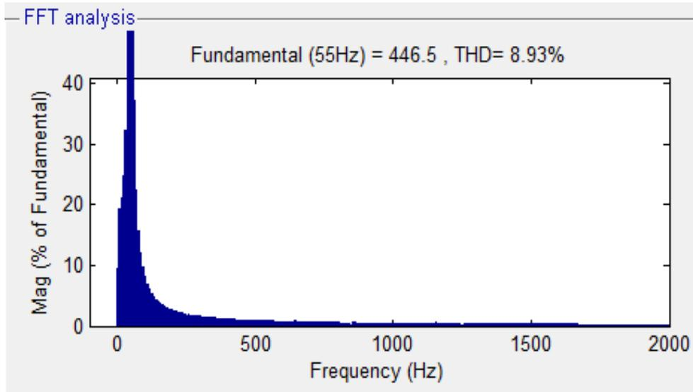
Figure 11: THD for NPC voltage using PI Controller
