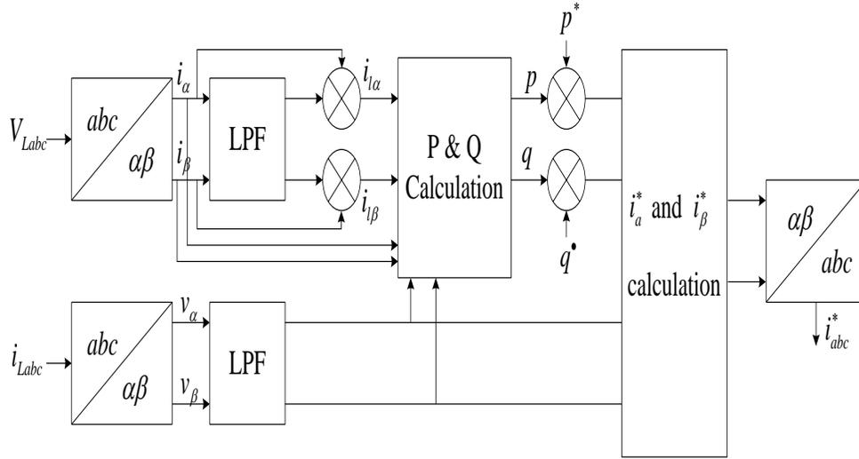
Figure 3: control structure of the shunt inverter
