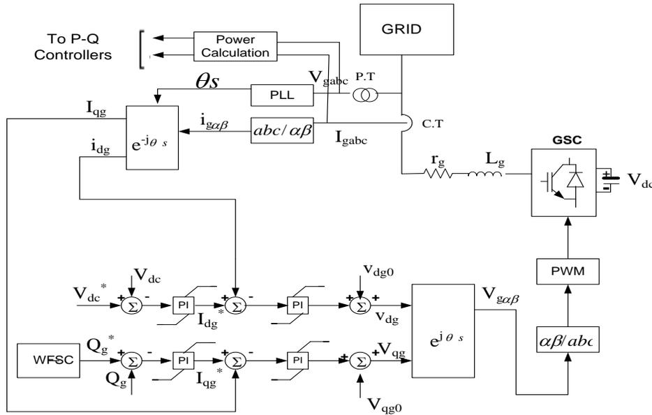
Figure 2: Structure of proposed PSO based GSC control diagram
