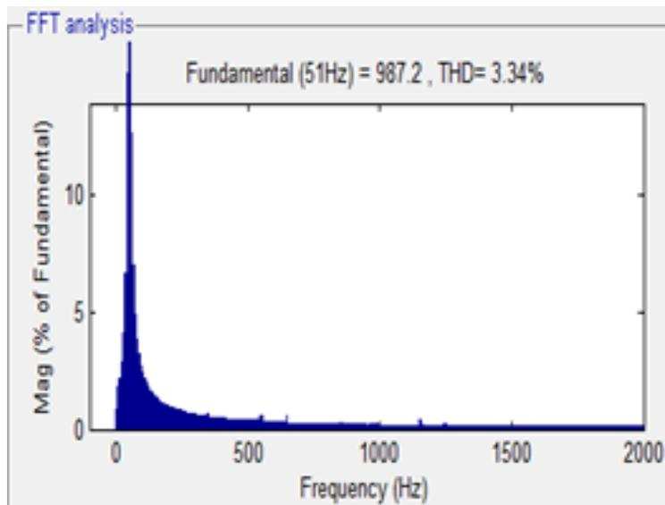
Figure 12: THD for NPC voltage using Fuzzy Controller
