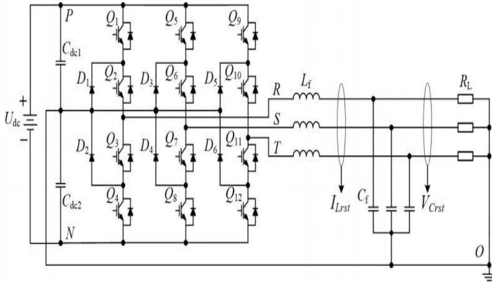
Figure 4: Topology of the NPC three-level inverter
