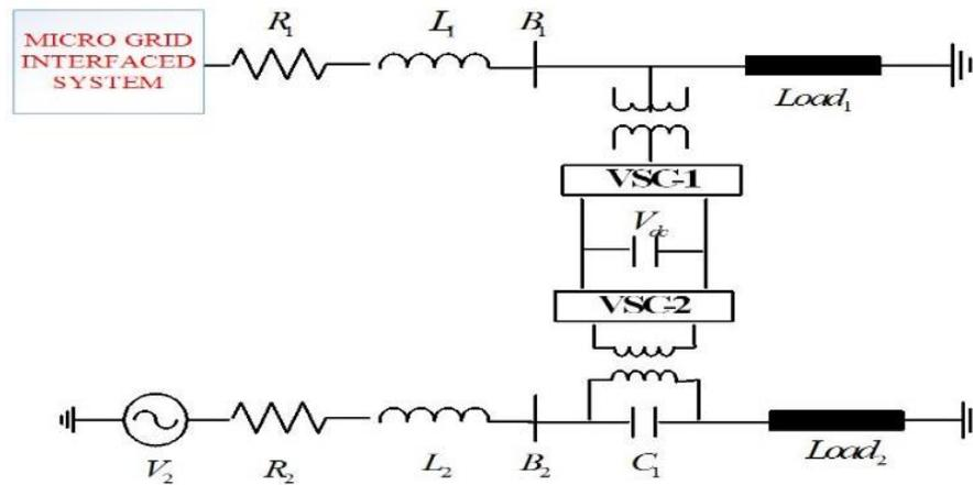
Figure 1: Structure of APF based Distribution System
