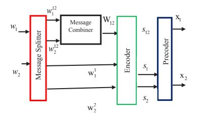
Figure 9. RSMA transmitter block for two users.
