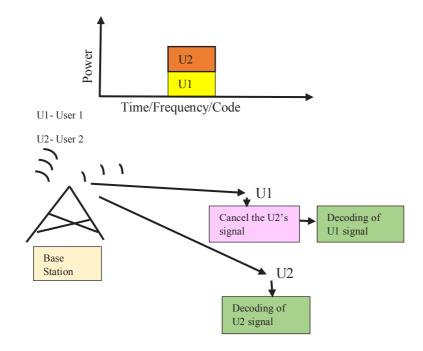
Figure 3. Basic NOMA principle in downlink communication with one base station two users.
