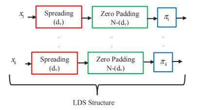
Figure 4. LDS structure for signature sequence generation.
