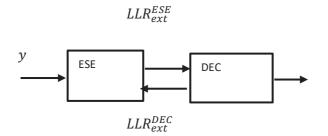
Figure 7. Iteration between ESE and DEC in IDMA receiver.
