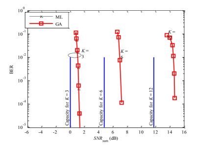
Figure 8. IDMA systems with EPC and SPC over AWGN channels. Rate-1/3 turbo coding followed by rate-1/2 repetition coding is used for each user with QPSK modulation [105].
