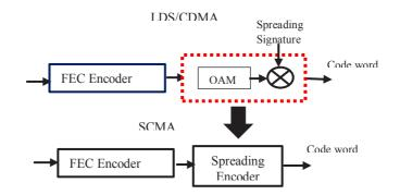
Figure 5. Merging of QAM and spreading to generate the SCMA code-word.
