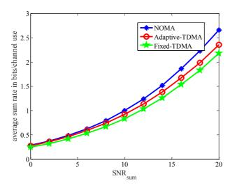
Figure 2. Achievable Sum rate of NOMA and OMA schemes under EEC. NOMA is based on SIC and Adaptive TDMA and Fixed length TDMA is considered as OMA (Jayashree, L. S. et al., 2021).
