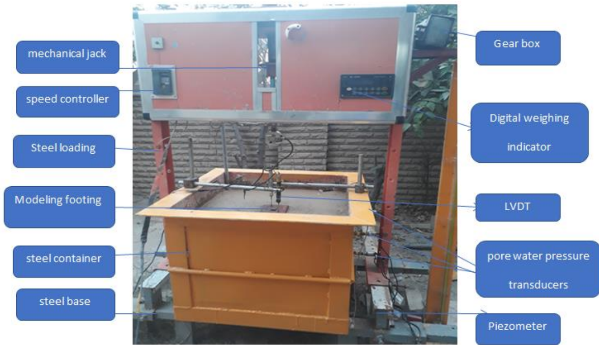
Figure 3. The physical model for static loading tests.
