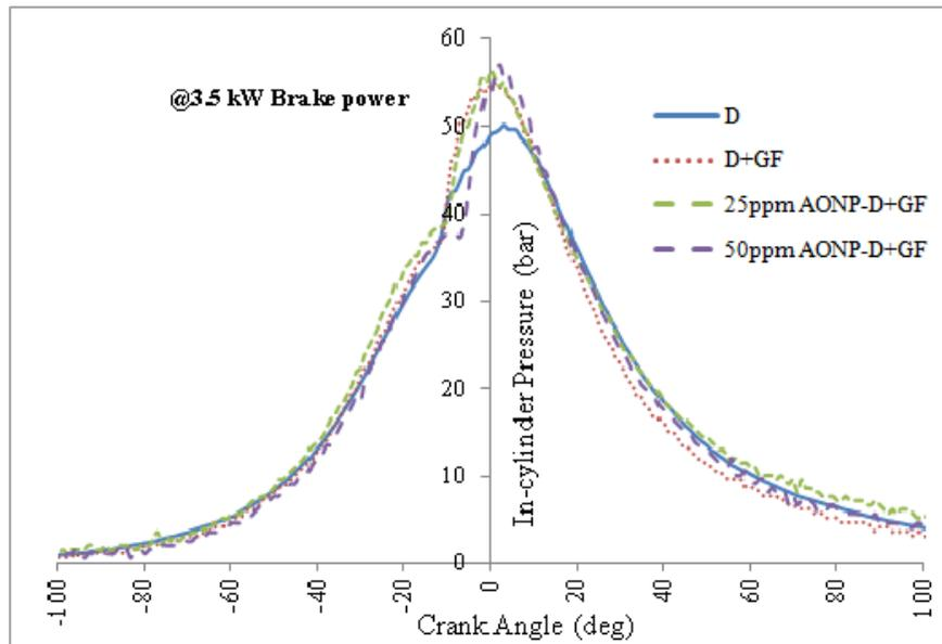
**Figure 8** Variations of In-cylinder Pressure with Crank Angle for different fuel blends
