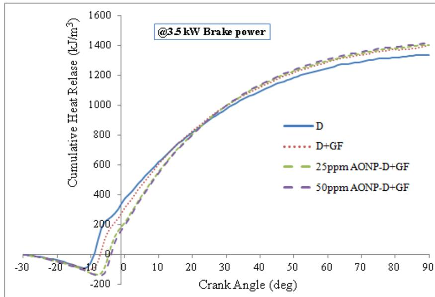
**Figure 9** Variations of Cumulative heat release with Crank Angle for different fuel blends
