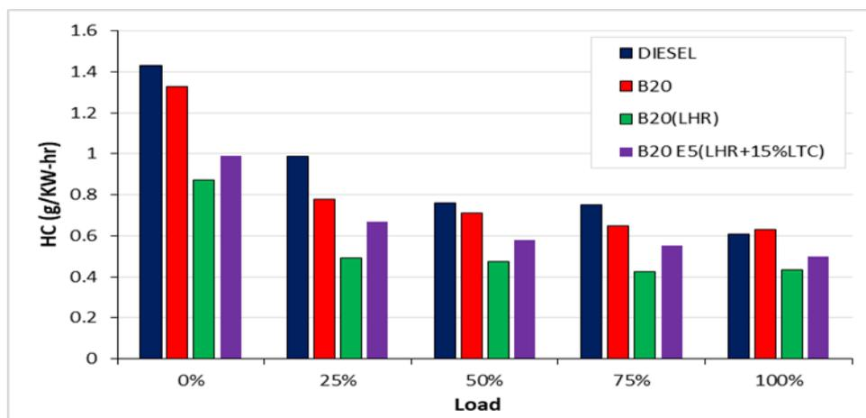
**Figure 12** HC Emission VS Load.
