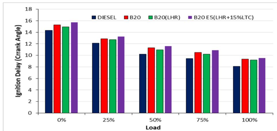
**Figure 11** Ignition Delay VS Load.
