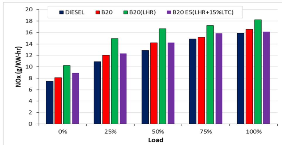
**Figure 14** NO<sub>x</sub> Emission VS Load.
