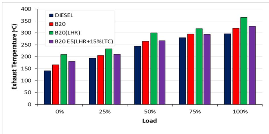
**Figure 8** Exhaust Gas Temperature VS Load.
