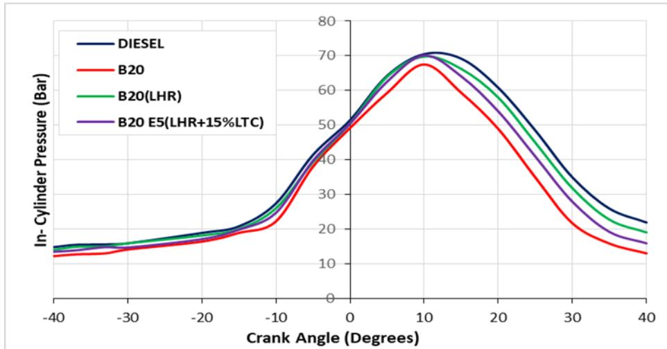
**Figure 9** In-Cylinder Pressure Vs Crank Angles.
