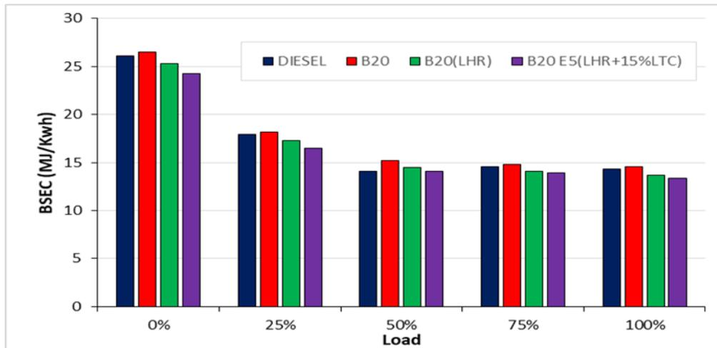
**Figure 7** Brake Specific Energy Consumption VS Load.
