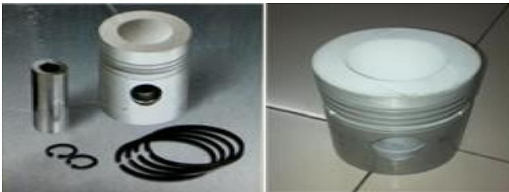
**Figure 3** Before and after coating of the piston crown.
