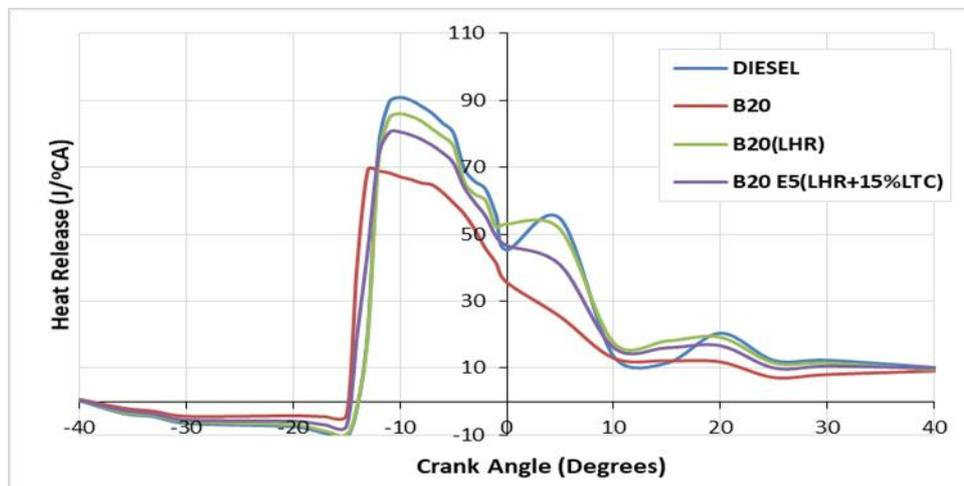
**Figure 10** Heat Release VS Crank Angles.
