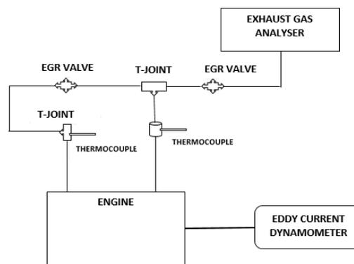
**Figure 5** EGR block diagram.
