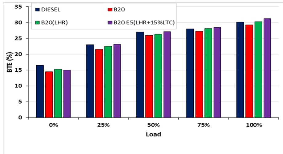
**Figure 6** Brake Thermal Efficiency VS Load.
