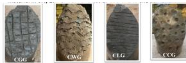
Figure 2 Surface preparation a) Grid b) waves c) lines d) chipped
