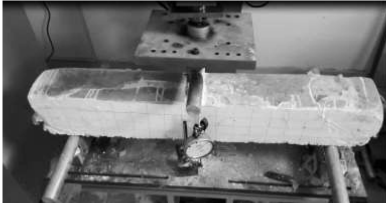
Fig. 3. Flexural bending test setup in three-point loading.
