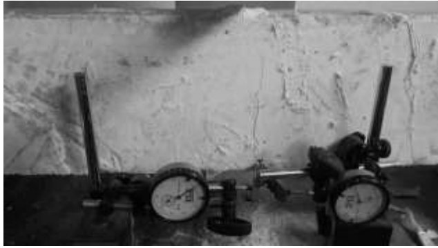
Fig. 10(a). Thin crack width of high volume fibre reinforced concretes specimens (DHS-7).
