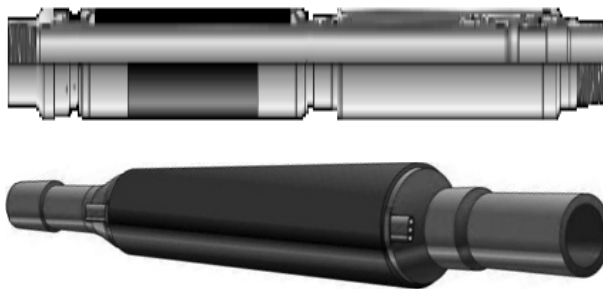
Fig. 1. Typical mechanical packer and swelling packer.
