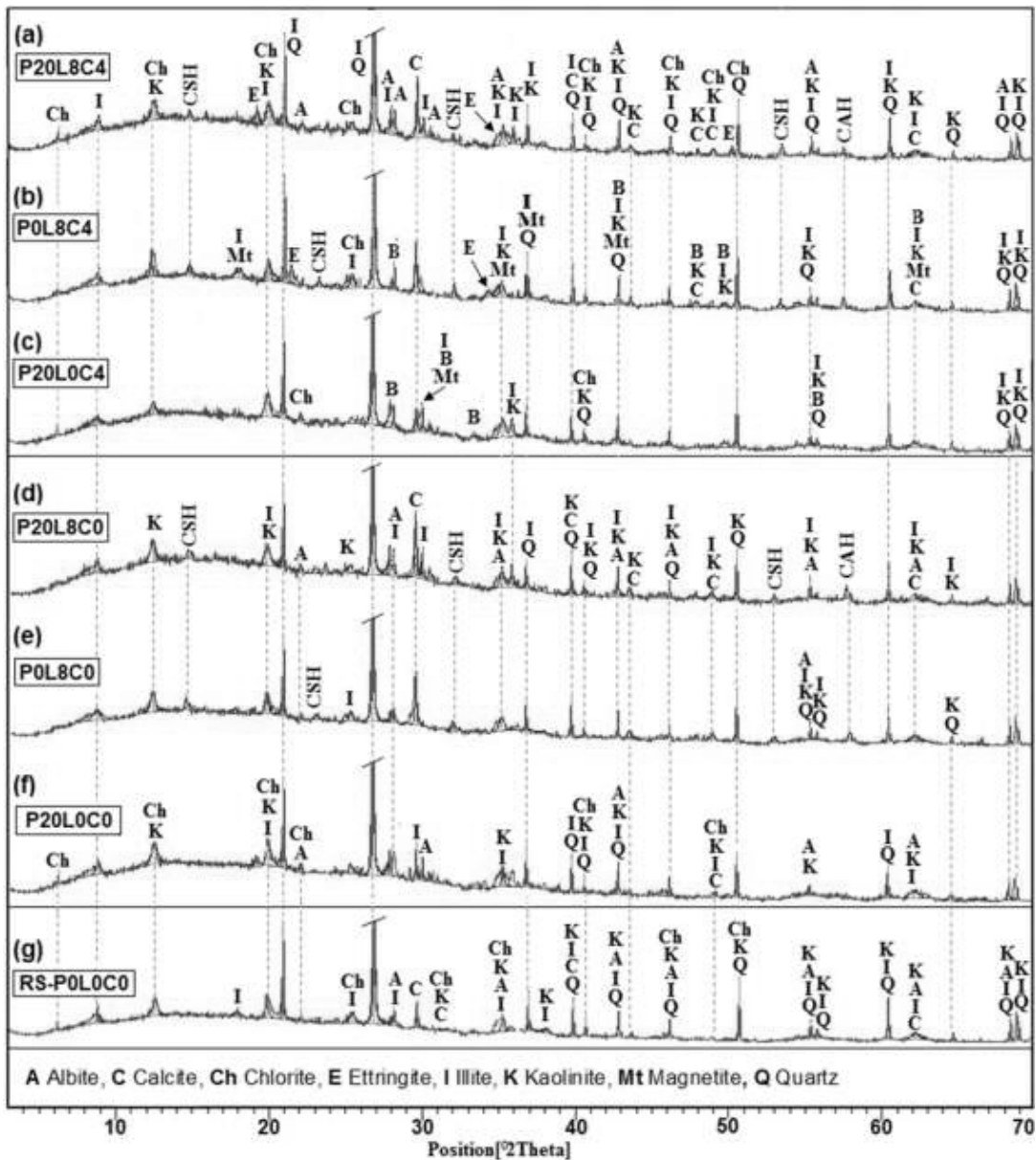
Fig. 10. XRD diagrams of the RS samples obtained after 60 days of curing period (a, b & c) treated RS samples containing 4% of \text{CaSO}_4 \cdot 2\text{H}_2\text{O} , (d, e & f) treated RS samples without \text{CaSO}_4 \cdot 2\text{H}_2\text{O} and (g) untreated RS sample without \text{CaSO}_4 \cdot 2\text{H}_2\text{O} .
