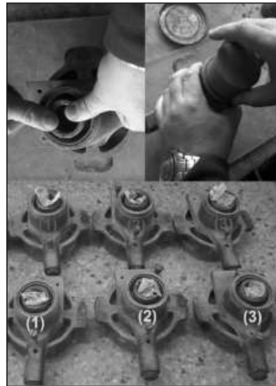
(b) Installation of the specimens in the shear box
