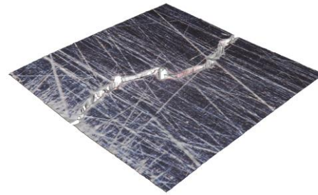
Figure 6: 3D surface of damaged specimen.
