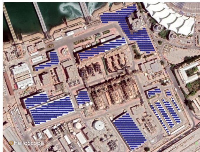
Figure 4: Satellite image of the Shuwaikh DP with the PV modules using HelioScope simulation.
