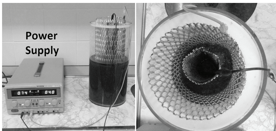
Fig. 2. The front and plan views of laboratory scale batch reactor
